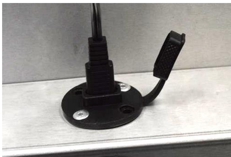
Charging Port with charging cable plugged in
